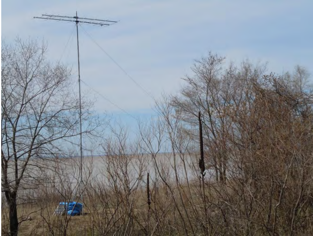
Figure 3. Automated tower and radio-signal receiver in place at Ottawa National Wildlife Refuge.
