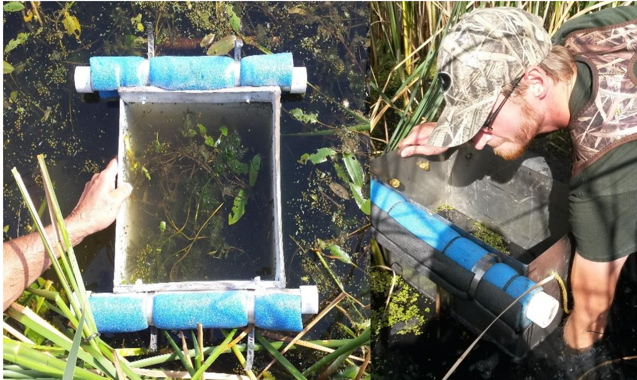
Figure 1. Sampling submerged aquatic vegetation with the modified Gerking Box Sampler.
